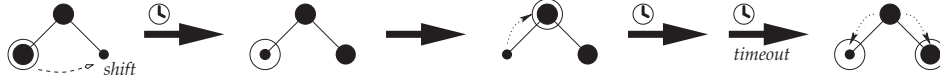
Fig. 5: The follow flag timeout. The follow flag is reset after a configurable timeout, to allow for finding newly heavily-hit children, to whom the collapse rule has previously been applied.
